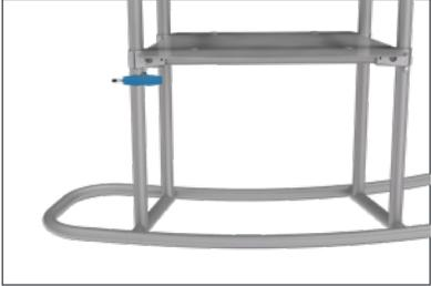
frame before tightening clamps down with hex tool.
