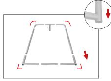
Step 6: Push banner stand frame onto posts of flat base or optional feet. Press evenly on both sides to make easier for the frame to go on.
