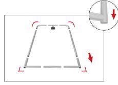
Step 6: Push banner stand frame onto posts of flat base or optional feet. Press evenly on both sides to make easier for the frame to go on.
