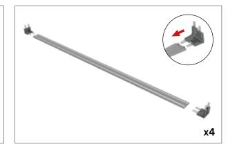
**Step 4:** Build the center power pole by push sections together. Slide on horizontal support clamp before attaching to frame. Important! Horizontal support clamp may be preinstalled. If not, center and tighten screw in Step 8.
