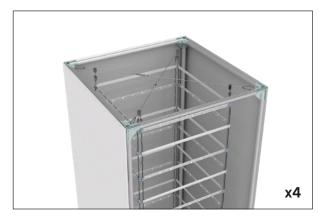
**Step 14:** Plug power supplies into the top of LED Light Arrays. 2 LED Light Arrays per power supply.
