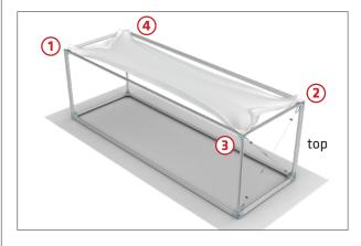
**Step 8:** Repeat Steps 6-7 until 3 sides are complete. Leave installation of fourth graphic until after the LED Light Arrays have been installed.
