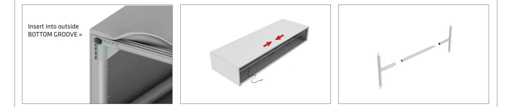
**Step 14: Turn. Position. Lock.** Insert tensioning pole into the bottom of display. Keep the pole flat until the entire pole fits inside the frame. **Turn** the pole 45°.
