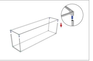
**Step 4:** At the top of the frame attach cable to left and right side. Tighten or loosen with hand pull.
