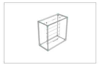
**Step 8:** Fit PVC inner boards onto the top of frame with wedge side face down. Position and align board until it fits down into the frame.
