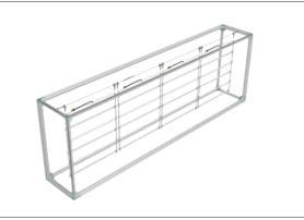
**Step 8:** Assemble center support brace by pushing and pulling together.
