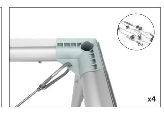
**Step 4:** Move to the center of cable and hand tighten turnbuckle to remove any remaining slack. Do not over tighten.
