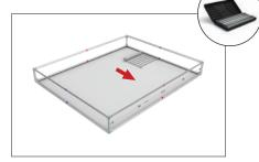
**Step 14: Turn. Position. Lock.** Insert tensioning pole into the bottom of display. Keep the pole flat until the entire pole fits inside the frame. **Turn** the pole 45°. **Position** and
