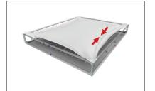
Step 10: Take out the LED Lights and gently unroll on the graphic with lights face down. WARNING! Do not drag lights across ground or it could break the LED lights.
