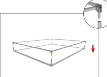
**Step 6:** Start in one corner of the frame and push the silicone edge of graphic into the inside groove. Insert for 4-6 inches in both directions. Repeat on all corners.
