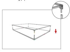
**Step 6:** Start in one corner of the frame and push the silicone edge of graphic into the inside groove. Insert for 4-6 inches in both directions. Repeat on all corners.
