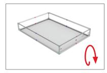
**Step 13:** Repeat Steps 6 and 7 to attch printed graphic for double -sided display or light block panel for single-sided display.
