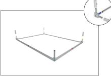
**Step 3:** Build two outer frames and connect top and bottom frames together in the corners with small connecting pipes.
