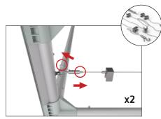
**Step 7:** Continue inserting silicone edge of graphic into the frame working towards the center of frame on each side. Do not over pull or stretch.
