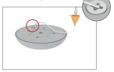
**Step 2:** In a clean, dry area, assemble the fabric onto the base by angling and tucking the silicone gasket into the bottom groove. **Step 3:** Flip base over carefully to prevent damage to graphic and repeat Step 2 for top groove.
