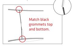
**Step 2:** Connect all corner sections to longer sections of the frame by matching shape symbols on pipes. Step 3: Align two frames together making sure holes face each other. Step 4: Push all support poles into one frame. Step 5: Locate all the poles pushed into black grommets and place one end of a cable eyelet over those poles.
