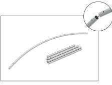
Step 6: Align top frame to bottom frame and push support poles into the frame. With some force connect the support poles in the
