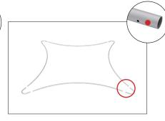
Step 7: Unzip print and place one frame inside. Position holes on frame to align with eyelets in graphic. Thread cable through eyelet. Repeat for all eyelets.
