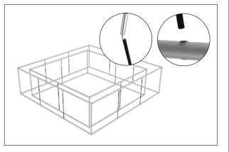
**Step 12:** Attach eybolts to the **bottom** of the larger hanging sign by screwing them lock into the 4 corners.
