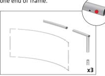
**Step 7:** Insert clamp pipe to bottom of frame. Insert clamp pipe into loop of cable before pushing into frame.
