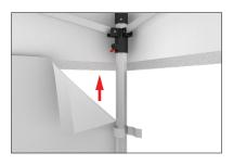
**Step 5:** Attach half wall to frame with Velcro strap just above push button lock. Repeat this front and back for each side wall.
