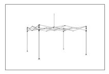
**Step 6:** Lift the 2 adjacent outer legs and slide out the inner legs until the button snap-locks into the hole of the outer leg. Repeat on opposite 2 legs until fully extended.
