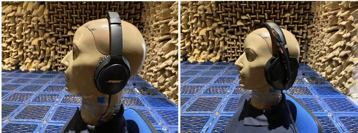
Figure 2a: Typical fit of BOSE (left) and N16 (right) headphones on HATS
