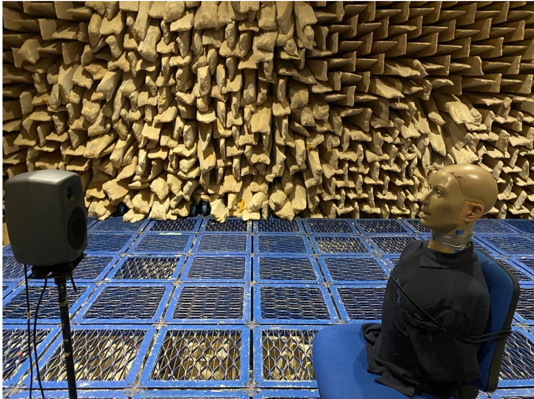
Figure 2b: Calmer Night fitted to HATS and the external source
