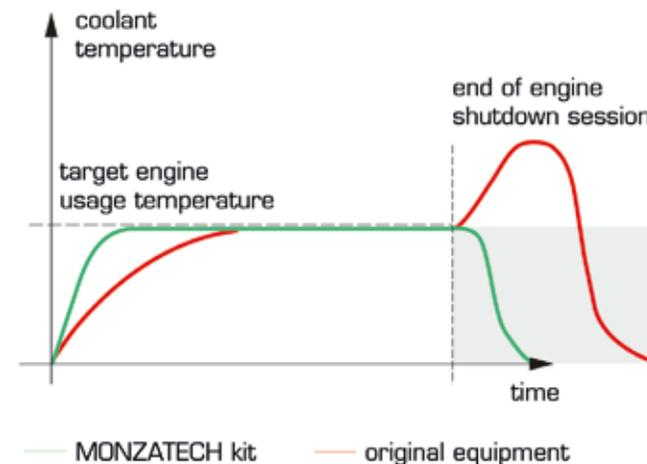
In This way, the fan can attend already at lower temperatures than those set by the manufacturer, avoiding a build-up of heat in the engine which is more difficult to disperse.
