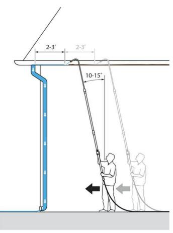
Best results will occur with regular maintenance of your gutters. The less the debris builds up, the quicker the cleaning time. If the gutter has been neglected for some time and is full of large twigs and fresh leaves, you may need to use the tip of the Guttermaster to try to flip the large pieces out of the gutter. Optional water flow brushes can be used with the Guttermaster pole for cleaning windows, siding, vehicles, and more. surfaces. То clean attach the appropriate brush for the task and
