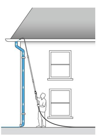
Stand back to one side (and not directly under the gutter) to avoid getting splashed. If the downspout is clogged, you may need to disassemble the downspout to clear the blockage. Once clear, turn the Guttermaster unit off and proceed to step number 2.
