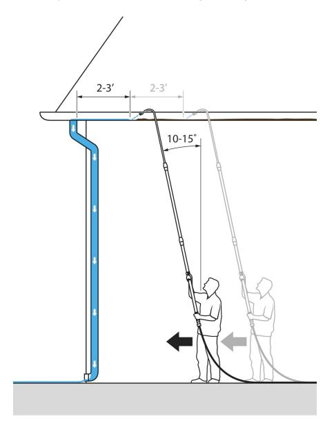
Please Note: Do not pull the garden hose along using the Guttermaster pole. It is recommended to leave plenty of slack in the hose while in use. To move to another area, pull the hose with one hand, while carrying the Guttermaster in the other.
