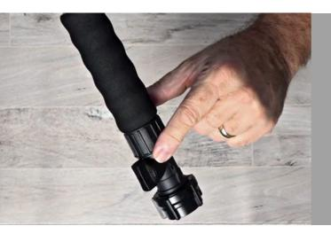
Make sure that the shut-off is closed, then attach your garden hose to the pole. Turn on the water flow at the tap. The Guttermaster pole is meant to generate a strong flow of water to push leaves and debris along your gutter, so don't extend it and turn it on full force right away.
