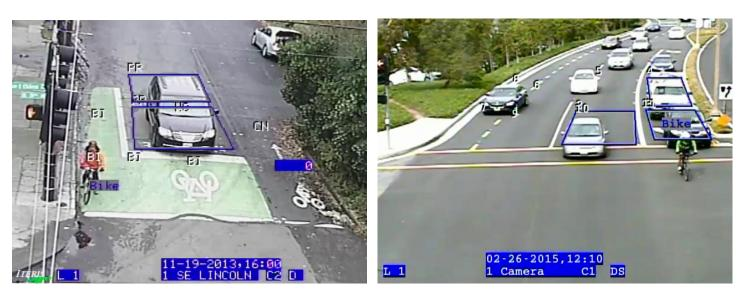
Bicycle zones are placed in bike lanes (left) as well as in vehicle lanes, including the left turn lane (right). Bicycles are detected and uniquely identified as "Bike" while regular motor vehicles are detected normally.
