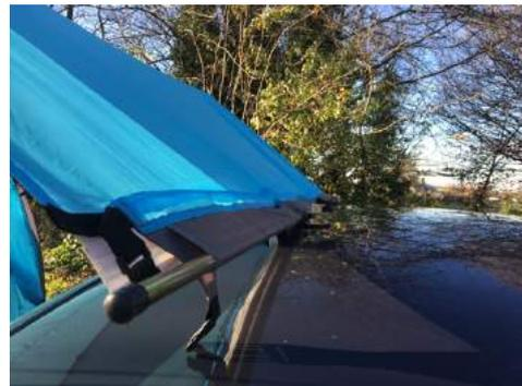
The suction clamp method is not ideal because sometimes the suction clamps loosens off (especially if it rains) and can come free. These have to also be purchased separately - <https://www.ebay.co.uk/itm/Adjustable-Brass-Suction-Awning-Canopy-Clamp-for-Vehicles-W-O-Rain-Gutter-C9050/152613878670?hash=item23887efb8e:g:MBoAAMXQhpdRpyYS>
