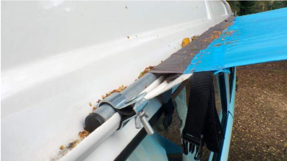
The last but not least preferable method is using suction clamps. There are three semi-circle gaps in the pole sleeve which allow for access onto the pole inside. The clamps attach onto the pole and then are suctioned onto the vehicle, either on the flat roof or side of the vehicle.
