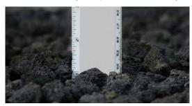
No more than 1" of media should cover the burner. Adding more may cause damage
