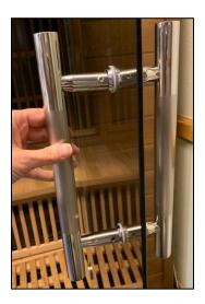
Using the hex screws provided with the handle, insert one small screw into the hole on the top cross section of the handle and tighten. Repeat for the bottom cross section of the handle. Move to the inside of the handle and repeat for the next two screws. It is normal for the hex screws to not sit flush to the handle.
