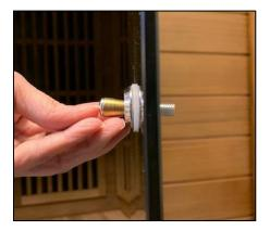
Add one plastic washer to the end of the screw now showing on the outside of the door. Place the remaining metal washer onto the screw with the flat side against the plastic washer. Repeat for the bottom hole.
