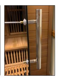
Place the inside portion of the door handle onto the upper and lower screw heads so that the handle fits into the recessed part of the metal washers. (Tip: It is helpful to have the hex screws already started in each of the four holes.)
