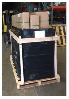
Break down the pallet at the delivery point and lay each box flat with the labeling facing up.
