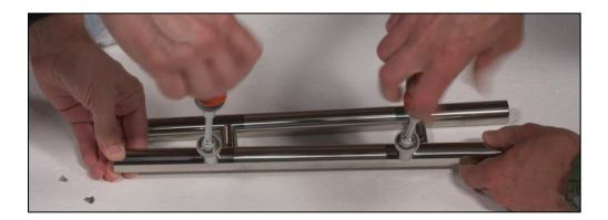
Included with each of the two screws are a metal cone, two plastic washers and two metal washers. Remove these items from the door handle keeping all but one metal washer and one plastic washer together.
