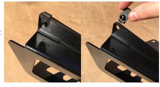
Press the gasket around the opening of the bumper.
