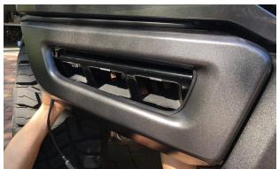
gasket. Before fully tightening be sure the bezel is aligned in the bumper hole and the gasket is seated evenly all around.
