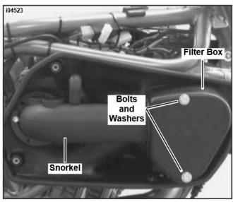
Figure 2. Remove Filter Box (S3 and S3T Shown)
