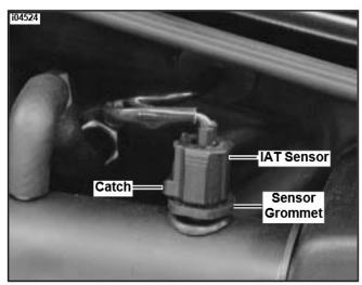
Figure 3. Remove IAT Sensor and Grommet (AII)
