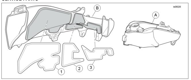
Figure 1. Buell 1125 Model Frame Insulation Kit
