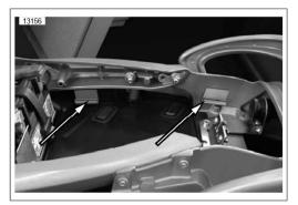
Figure 3. Extension Cord Retaining Clips
