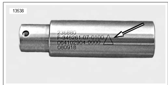
Figure 8. Triangle Marking on Cam Chain Tensioner
