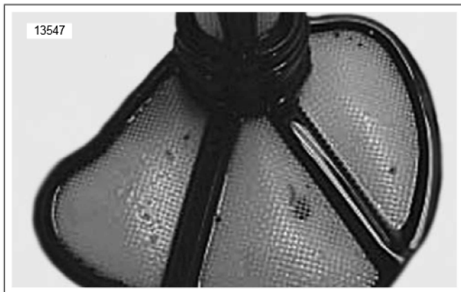
Figure 1. Oil Strainer: Acceptable Small Particles
