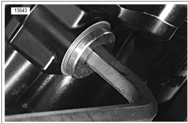
Figure 6. Remove the Tensioner Plug
