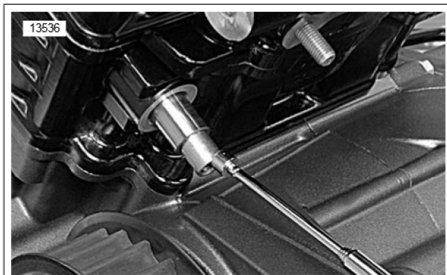
Figure 7. Remove the Chain Tensioner
