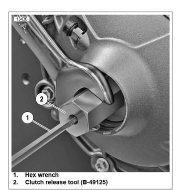
Figure 4. Removing Spherical Nut
