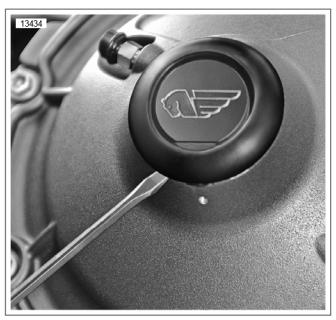
Figure 1. Secondary Clutch Actuator Cover Plug
