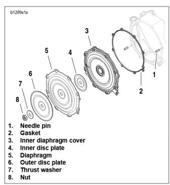
Figure 14. Diaphragm Assembly
