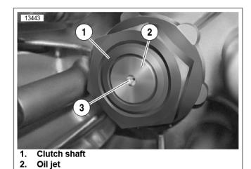
Figure 12. Installed Oil Jet
