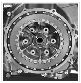
Figure 9. Clutch Shaft Bore
