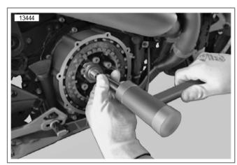
Figure 11. Oil Jet Installation
