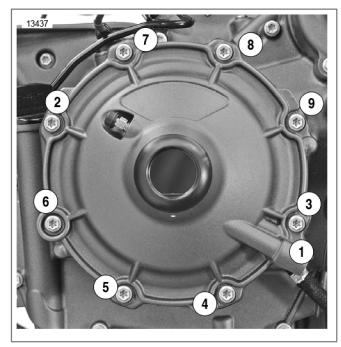
Figure 5. Secondary Actuator Cover Torque Sequence
