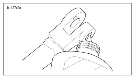
Figure 4. Threaded Area for Loctite Application
