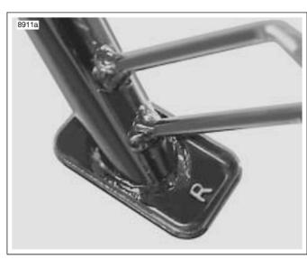
Figure 1. Correct Sidestand with Footpad Stamped
