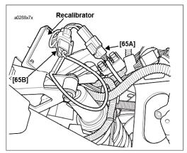
Figure 4. Connecting Recalibrator
