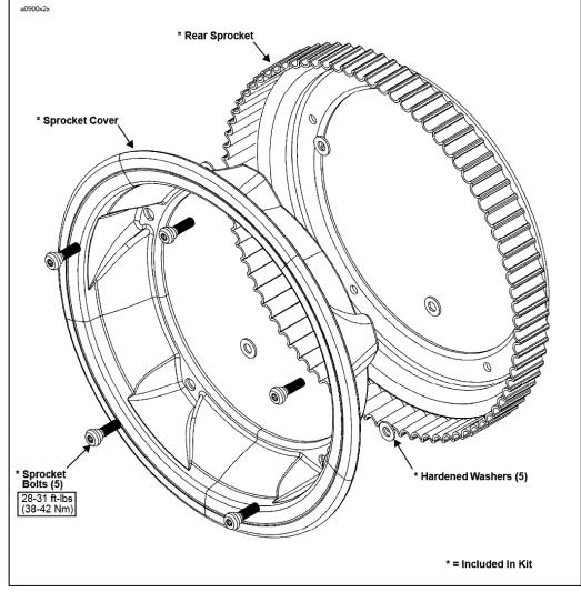
Figure 3. Rear Sprocket Assembly
