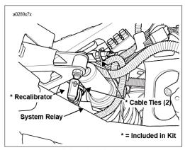
Figure 6. Securing Wire Harnesses
