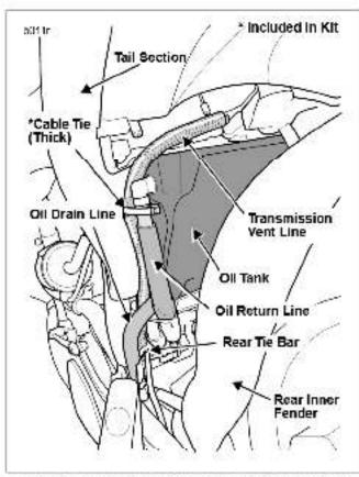
Figure 7. Transmission Vent Line Routing (Rear View)
