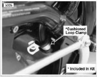
Figure 3. Loop Clamp Orientation Before Installation
