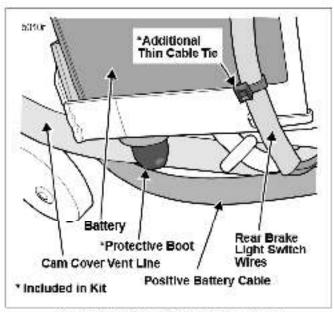
Figure 6. Positive Battery Cable Routing
