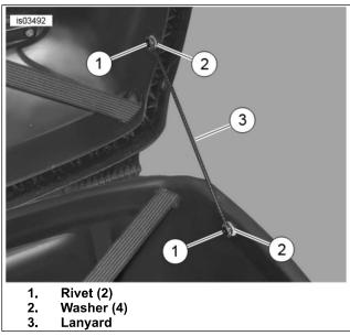
Figure 1. Remove Existing Parts
