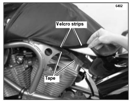
Figure 1. Line up protective tape underneath velcro strips.
