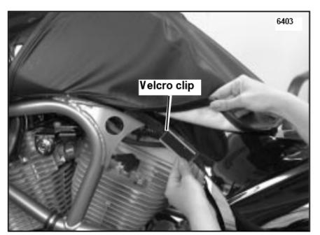
Figure 2. Install velcro clips over protective tape.
