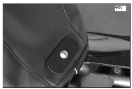
Figure 3. Secure tank mask to bike with screw.
