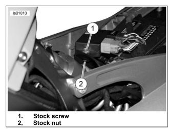
Figure 1. Remove Stock Screw and Nut
