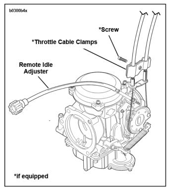
Figure 1. Carburetor Assembly
