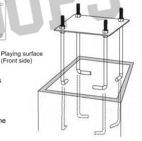
YOU ARE NOW FINISHED WITH THE INITIAL ASSEMBLY STEPS. DO NOT PROCEED WITH THE REMAINING ASSEMBLY UNTIL THE CONCRETE HAS FULLY CURED. CURING WILL TAKE A MINIMUM OF 5-7 DAYS. IN HUMID CLIMATES OR WET WEATHER, ALLOW ADDITIONAL TIME FOR THE CONCRETE TO CURE.
