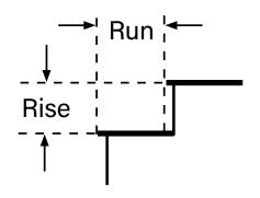
Measure the rise and run as shown, and use the table to determine the stair angle in degrees.
