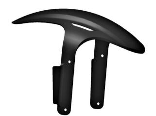
These parts are handmade of fiberglass come with a black gelcoat finish. This coating is not final use coating and will need to be top -coated (such as paint) for final use. Minor surface imperfections and scuffs are normal and may happen during taking parts out of the mold and shipping. This is allowable as the coating will need to be scuffed for final top-coat preparation.
