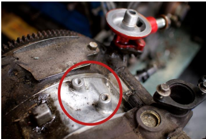
Image 3: Recommended engine grounding location
