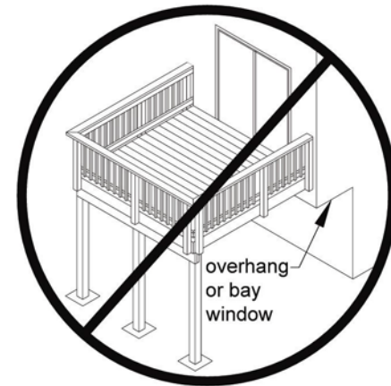
Figure 18. No Attachment to House Overhang
