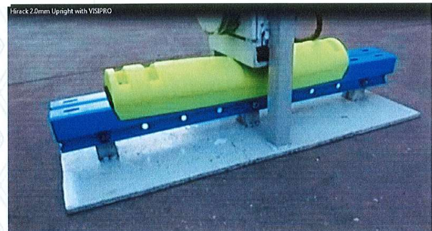
This photo shows the VISIPRO during the impact. Note the deflection of the VISIPRO as the impact force is absorbed.
