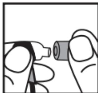
1. Remove the silicone tip from the earphone.
