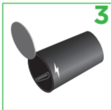
rotate the now loose backplate away from the earphone so it allows you to easily plug the USB cable
