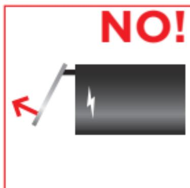
**WARNING:** Do not pull the backplate up to plug the USB cable, this may damage your headset. Always rotate the backplate away from the base to charge.
