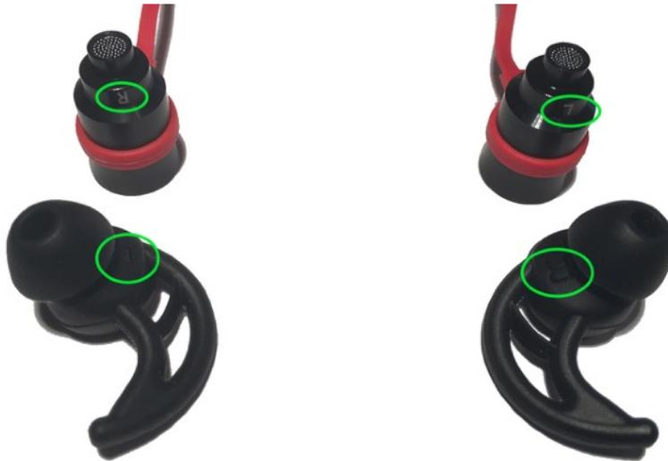
**5.** Now you may adjust the length of the cable so it rests comfortably on the back of your head. Please note, when set up correctly, the winged earphone tips must point towards the cable. The final setup looks like this:
