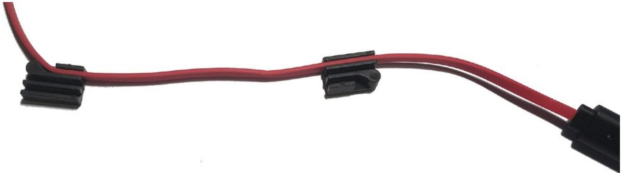
**2.** Now wind the cable around the rounded corner of the left management clip and straight through the one on the right:
