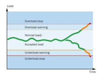
Emotron softstarters and shaft power monitors offer protection from unnecessary downtime, energy loss and equipment damage. Warning and safety stop levels are easy to set.
