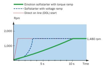
The built-in torque control enables you to start smoother with constant acceleration. This means improved process control and lower maintenance costs.
