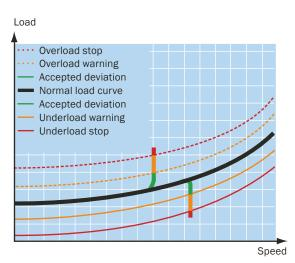
Emotron variable speed drives adapt the pressure/flow to the level required. Deviations from normal operation are quickly detected over the entire speed range, thanks to the unique load curve protection (patent pending EP 05109356).
