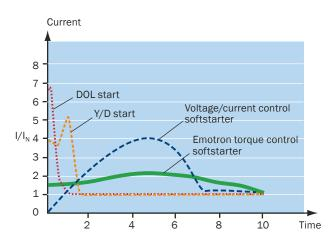
Start current is greatly reduced with the Emotron softstarter. You can use smaller fuses and cables and thus benefit from reduced installation and energy costs.
